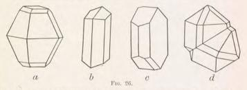
a represents an Orthorhombic crystal of sulphur. Other crystals of this system are shown in Figs. 31 and 54. b represents a Monoclinic crystal, and c a Triclinic crystal. d is a crystal of the Tetragonal system, which has the appearance of having been cut across and one-half revolved through an angle of 180° on the other half. Such crystals are known as twins, and are of not uncommon occurrence, e.g., twin octahedrons. On a following page a figure of a twin crystal of feldspar is shown.
